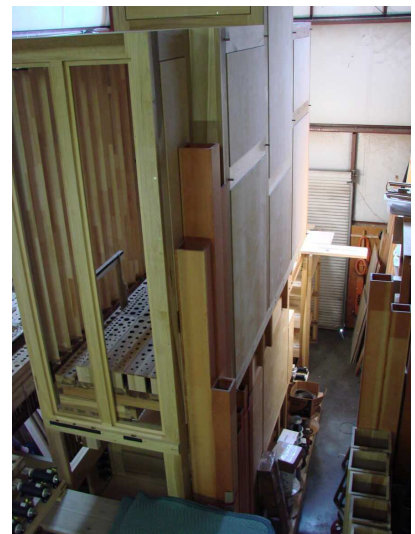
The swell box of St George's new organ at the Richards Fowkes' factory
